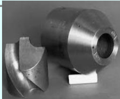
Swirl cone liquor gun and firing Pattern
